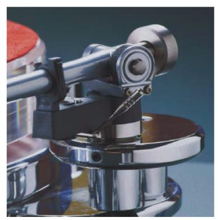
controls the arm's freedom of movement. The main counterweight is off-center to enable horizontal balancing. With a small supplementary weight the bearing load can be adjusted. The head shell is only slid on to the arm shaft and
